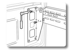
4. With the 10mm wrench, remove two bolts connecting the rail with the door.
